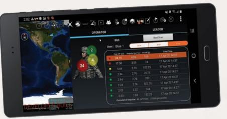
**Mobile Connectivity:** The Blast Gauge System App (BGSA) for AndroidTM and the Android Team Awareness Kit (ATAK) allows for near real-time data analysis and download with Bluetooth 4.1.
