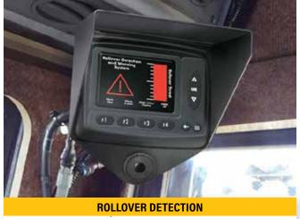
Audible Alert Options External buzzer up to 110 db Output for intercom systems
